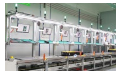
03 Inverter intelligent assembly line
