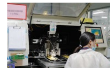
02 AI automatic horizontal plug-in machine 01
